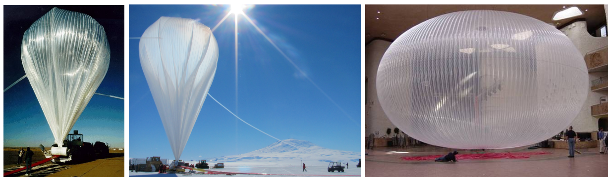
Figure 2.3: From left to right: a conventional balloon launches from Ft. Sumner [20]; an LDB flight commences in Antarctica [10]; a ULDB is tested in a hangar [14].
