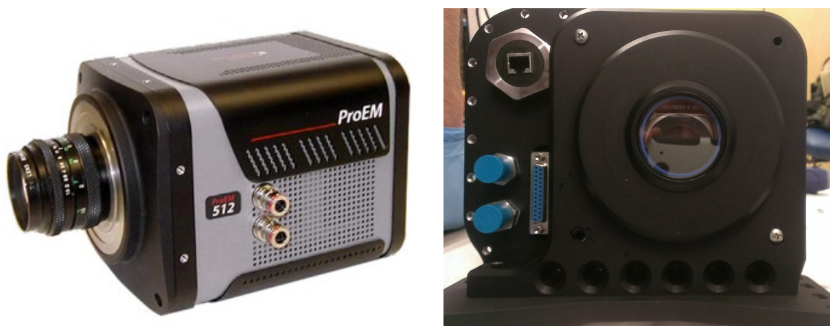
Figure 2.14: The science camera is a ProEM scientific CCD from Princeton Instruments. On the UV-VIS bench, it is mounted within a pressure vessel with a power port, an ethernet passthrough for data transfer and a UV-enhanced window.
